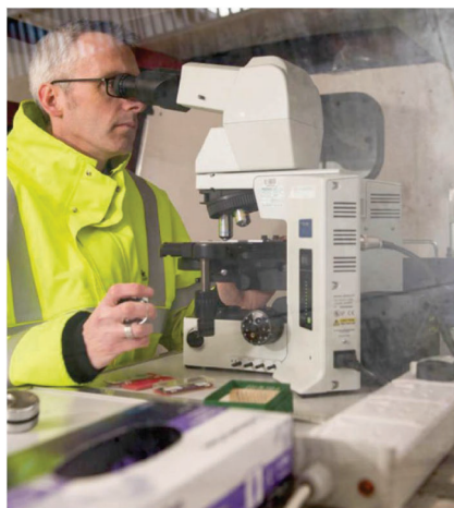
Figure 5.3 Analyst carrying out analysis by phase contrast microscopy in a mobile laboratory
